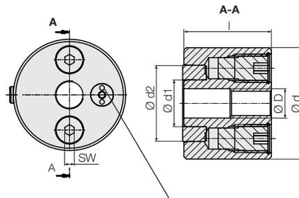
Projection of the indicator pin of the optical clamping force indicator when the nominal clamping force is reached:
