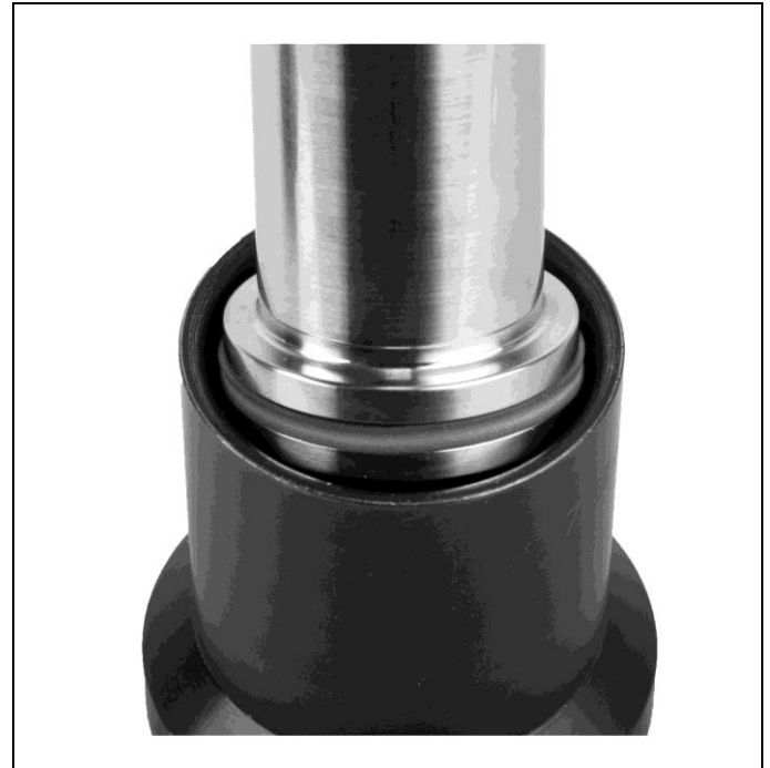
Figure 8: Calibration of an exterior seal by means of a tool.
