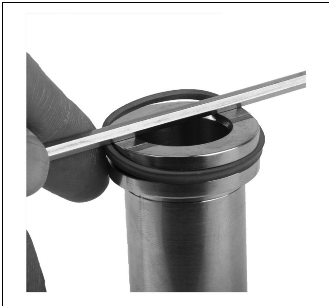
Figure 7: Mounting in a closed slot without assembly aid.
