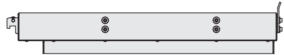
The rollers are lowered during transport. The die rests securely on the platform.
