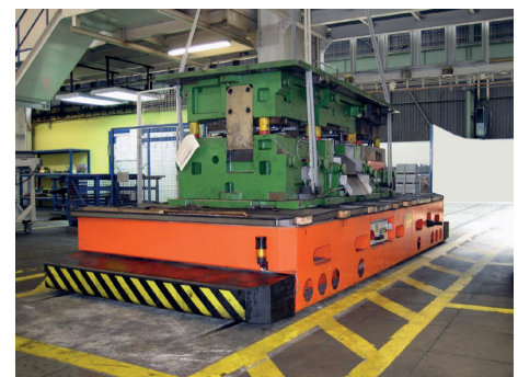
Transport cart, movable on rails
